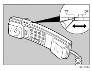
The switch on the handset should be in the appropriate position-TT (Tone Dialing) or DP (Pulse Dialing).
